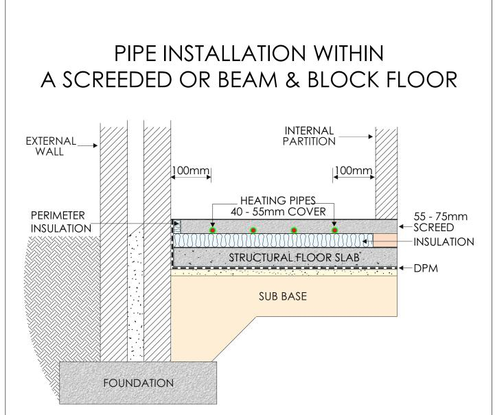
This technique is preferred by many builders. A concrete sub-base is poured and the construction of the house may then continue right up to second fix before the pipes need to be installed. **100mm** minimum **high density** extruded polystyrene insulation is used. The pipes are attached to the insulation and a minimum 60mm concrete screed is poured around the pipes to give at least 40mm cover over the pipes. This gives good thermal conductivity with a good response time for the end user.
